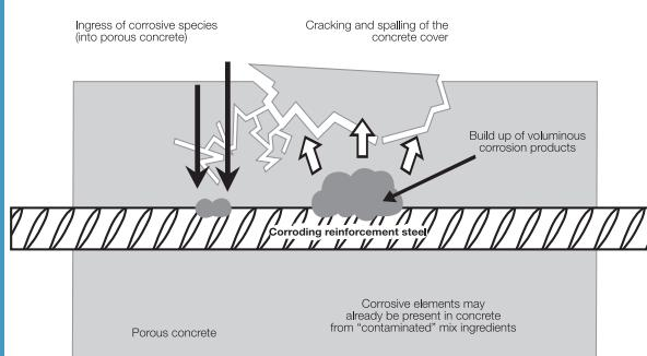
Corrosion of metal is natural and rapid in areas with high humidity, seacoasts, high salinity, etc. This menace can destroy even the toughest buildings, bridges, dams, chimneys, plants, ports etc. The corrosion process can be broadly explained as follows:
